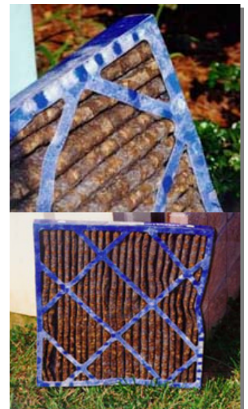
Moisture damage and microbial growth on pleated filters.
